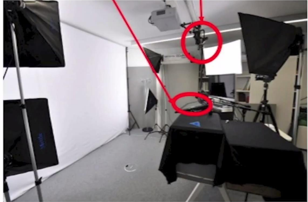
Screen recording of the content (fiducial markers on the tablet)
